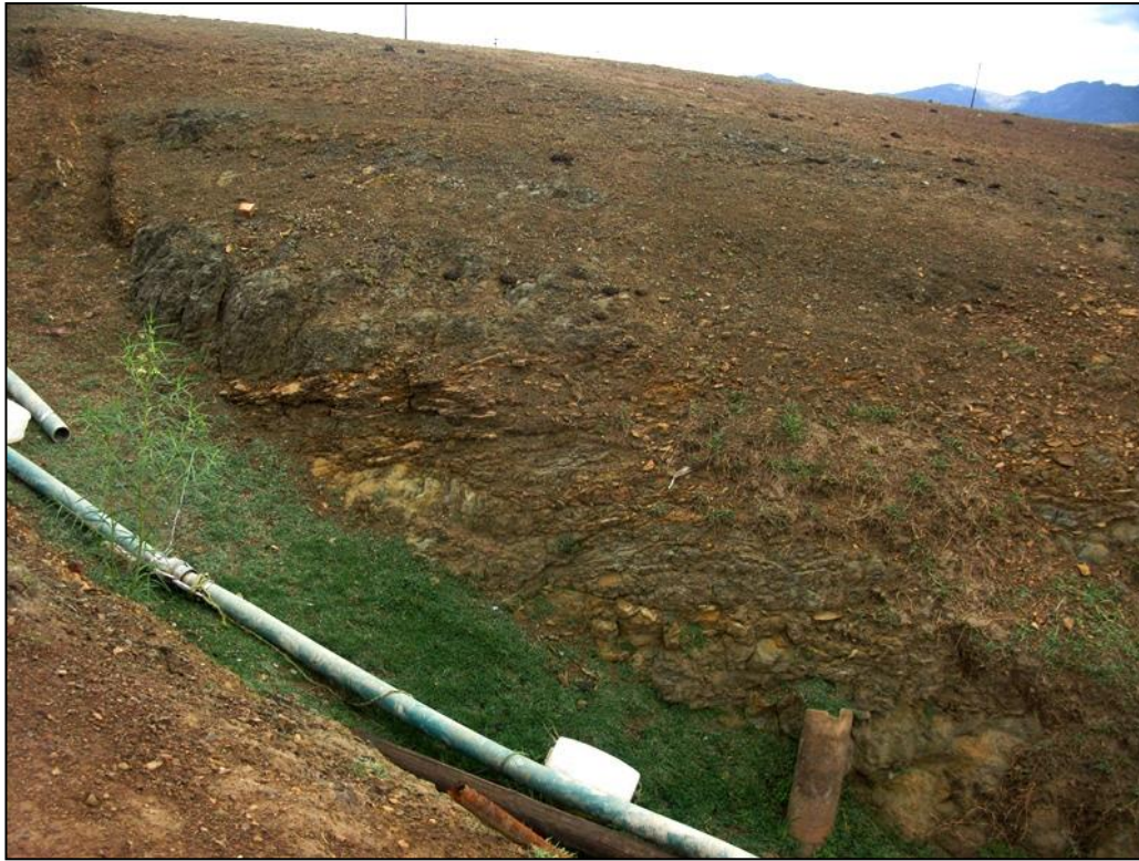
Figure 7. Highly fractured, faulted & weathered Voorstehoek Formation bedrocks exposed in a short pipeline trench on the southern edge of the existing dam (Source Almond, 2018).
