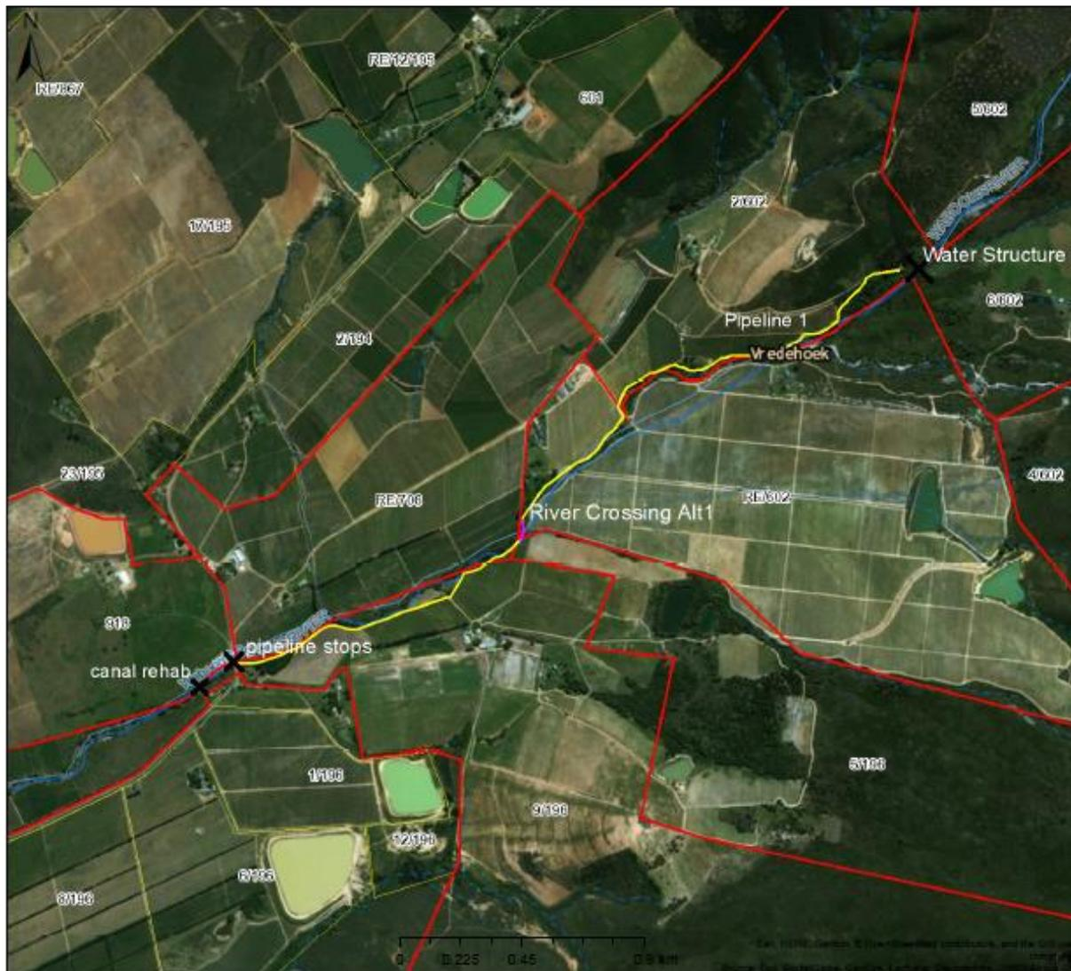
**Figure 3: The proposed pipeline in relation to existing farm boundaries (red)**
