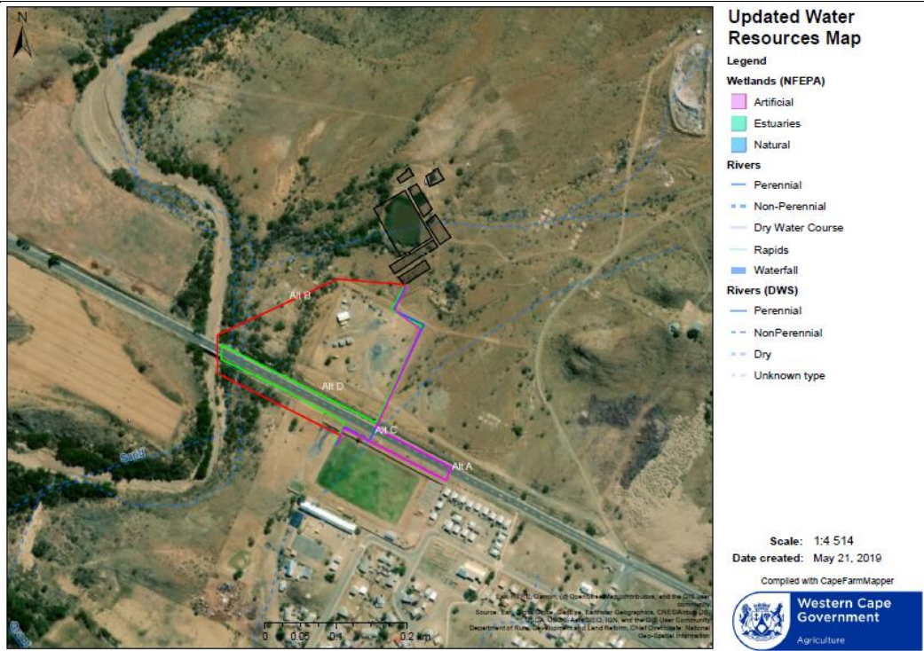
Figure 6: Water Resources Map indicating the proposed layout if the WWTP upgrade as well as pipeline alternatives (Cape Farm Mapper, 2019)
