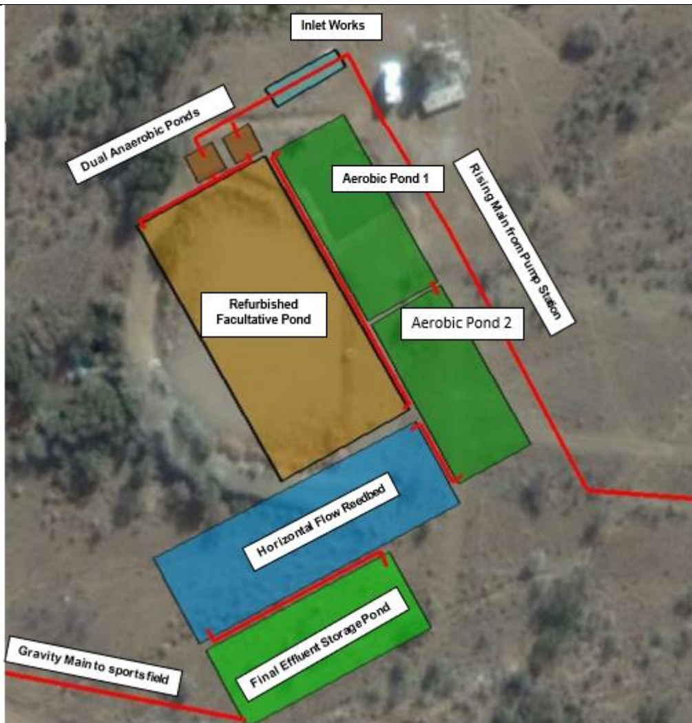
Figure 2: Proposed layout of refurbishment and improvement works of Klarstroom WWTW (BVI Technical Report)
