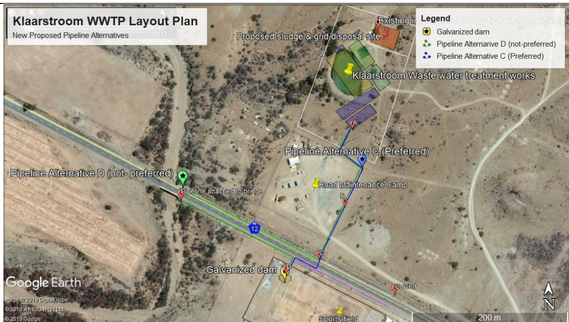
Figure 4: New proposed pipeline alternatives. Alternative C, blue line, is considered the new preferred alternative. It is proposed this route cross the N12 by means of horizontal directional drilling. Alternative D is also considered, the proposed pipeline to follow the route of Alternative A and C up until point C, to remain mostly within the N12 road reserve and to cross the N12 attached to the existing bridge.
