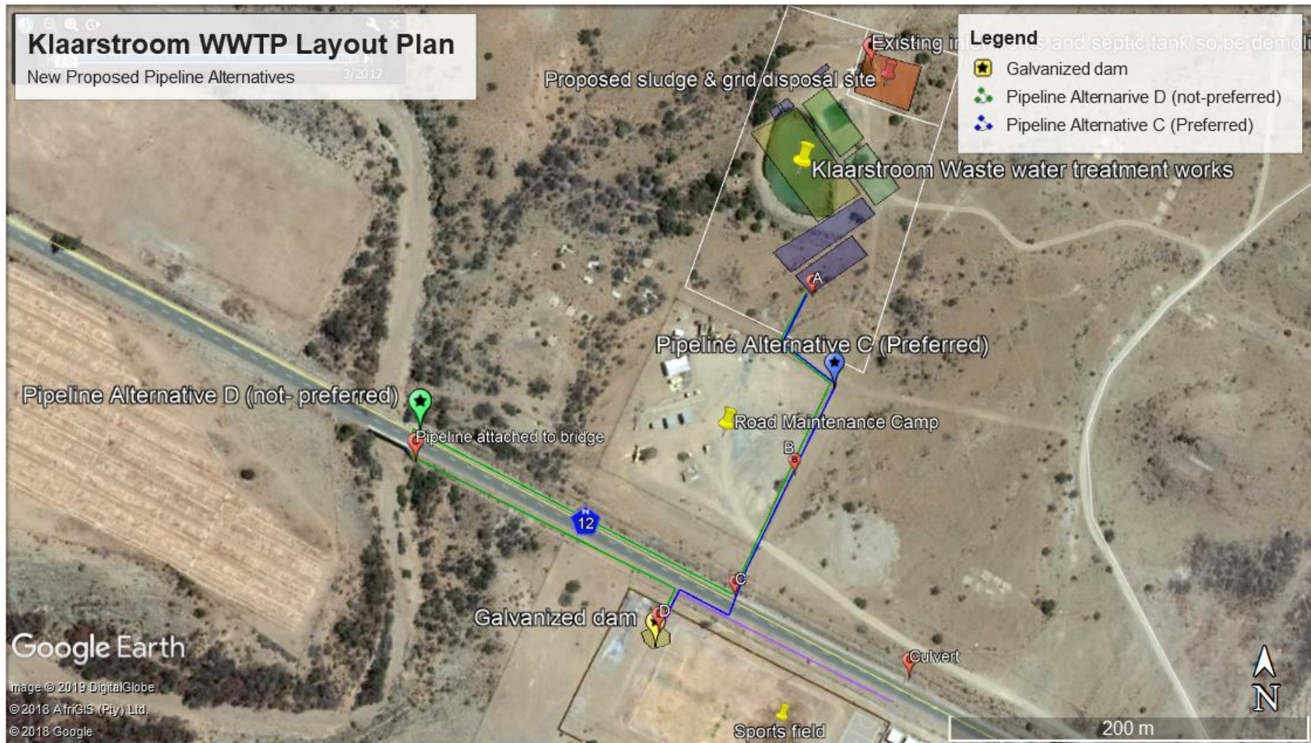
Figure 7: New proposed pipeline alternatives. Alternative C is considered the preferred alternative. It is proposed the pipeline cross the N12 by means of horizontal directional drilling. Alternative D was also considered, the proposed pipeline to follow the route of Alternative A and C up until point C to the north of the N12, from here it is proposed the pipeline follow the N12 road reserve to the existing bridge to the west. The pipeline to cross the N12 over the bridge. Pipeline to follow the road reserve to the south of the N12 where it will terminate in the proposed dam on the sports field.
