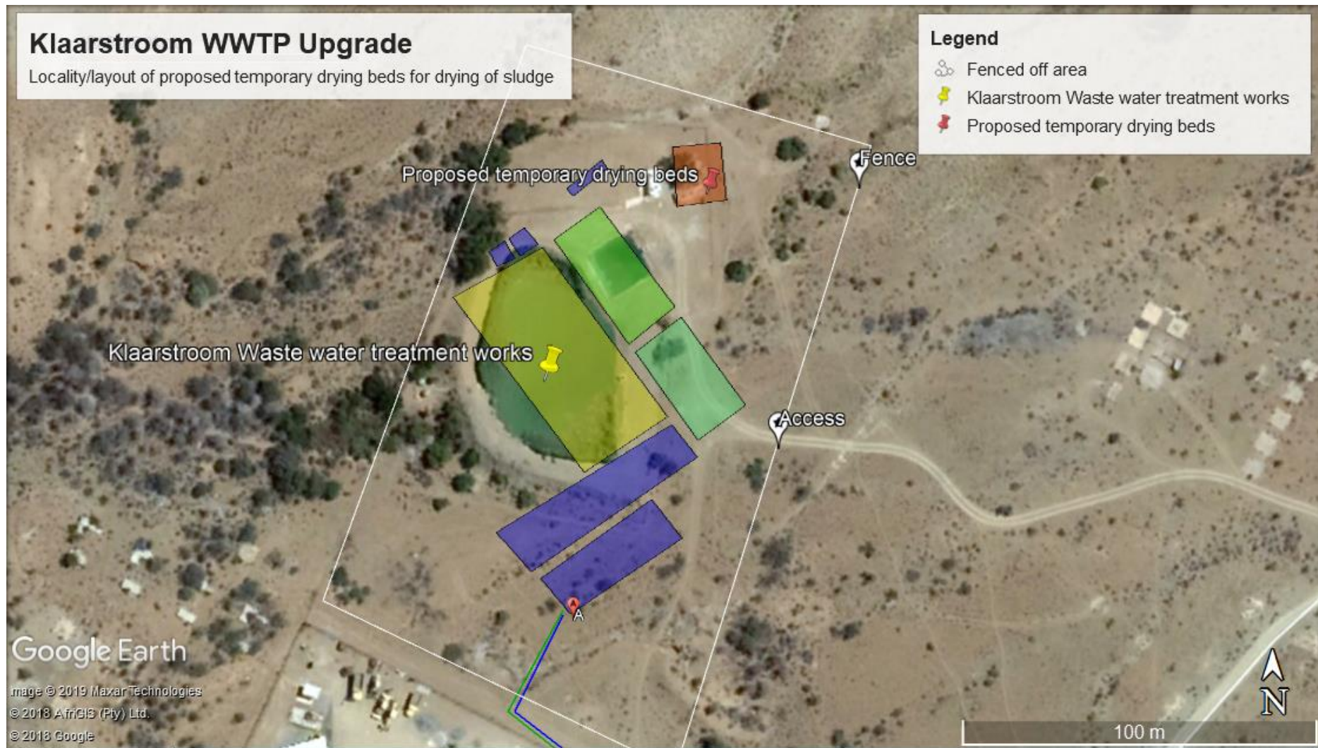
Figure 8: Locality map indicating the locality and layout for the establishment of temporary drying beds (250m 2 ) on disturbed land.
