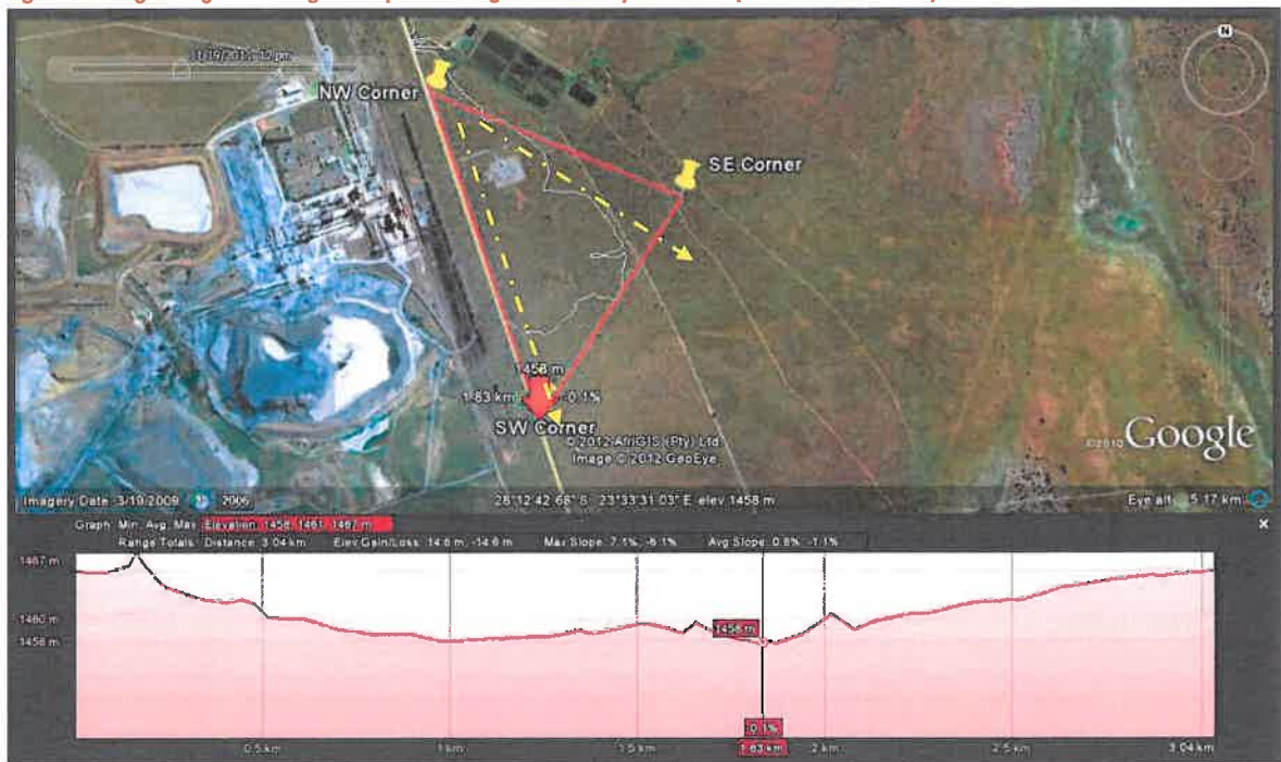
Figure 5: Google image indicating the slope following the boundary of the site (direction NW-SE-SW).
