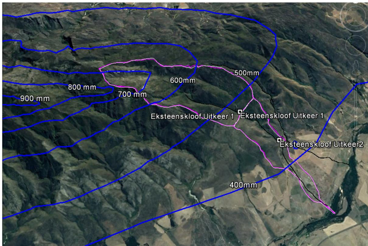
3. The WR2012 software was configured to produce the total flow of the Eksteenskloof at the confluence with the Riviersondered as well as at the upper and lower diversion sites.
