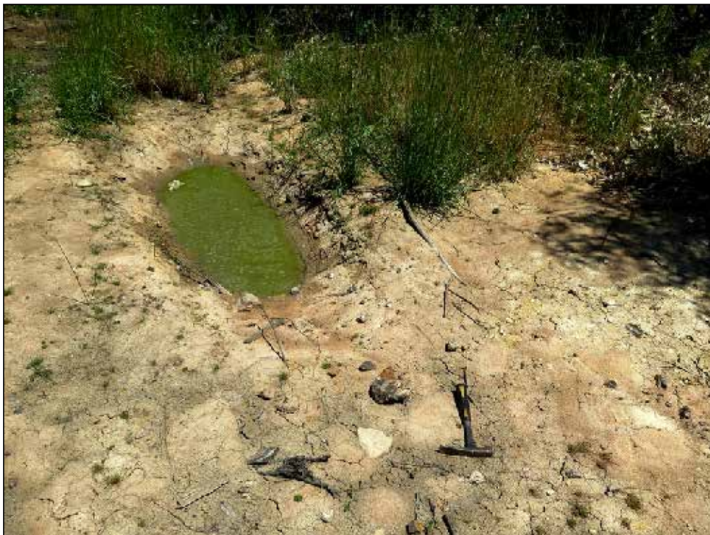
Figure 7. Test-pit area showing pale sandy soils with sparse, dispersed gravels of rusty sandstone, kaolinitised granite, weathered Tygerberg Formation wackes and quartzites as well as pale calcrete (Hammer = 30 cm).
