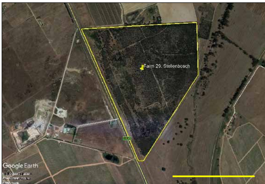
Figure 2. Google Earth© satellite image of Farm 29 Calcutta located on the eastern side of the R304 tar road c. 8.75 km NW of Stellenbosch showing the almost flat-lying terrain overgrown with eucalyptus and acacia trees with no obvious bedrock exposure. Pale bedrocks – probably clays derived from weathered Malmesbury Group metasediments – are
