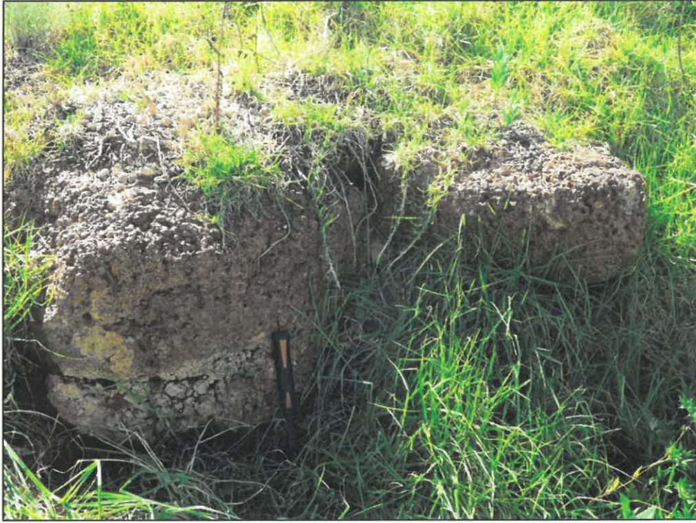
Figure 10. Thick ferricrete hardpan exposed in the wall of a drainage ditch, southern sector of Louw's Bos 502 (Hammer = 30 cm).
