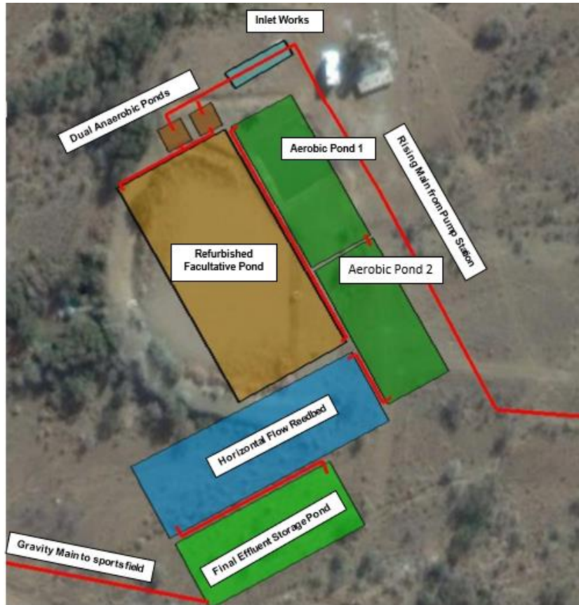
Figure 2: Proposed layout of refurbishment and improvement works of Klaarstroom WWTW (BVI Technical Report)
