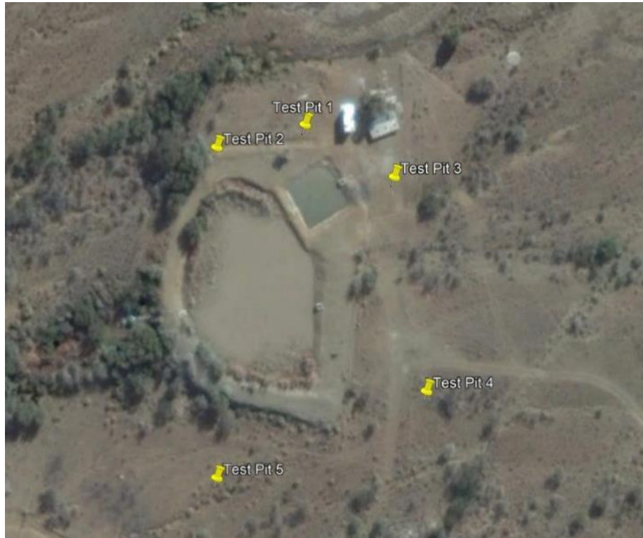
Figure 11: Position of test pits for geotechnical investigation
