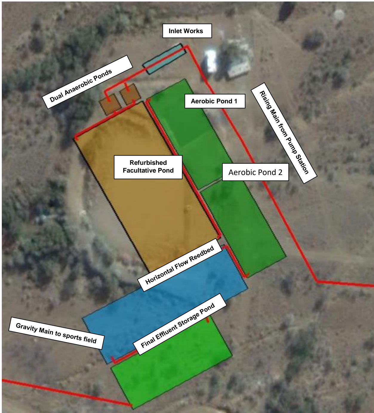
Figure 9 New Klaarstroom WWTW (BVi)
