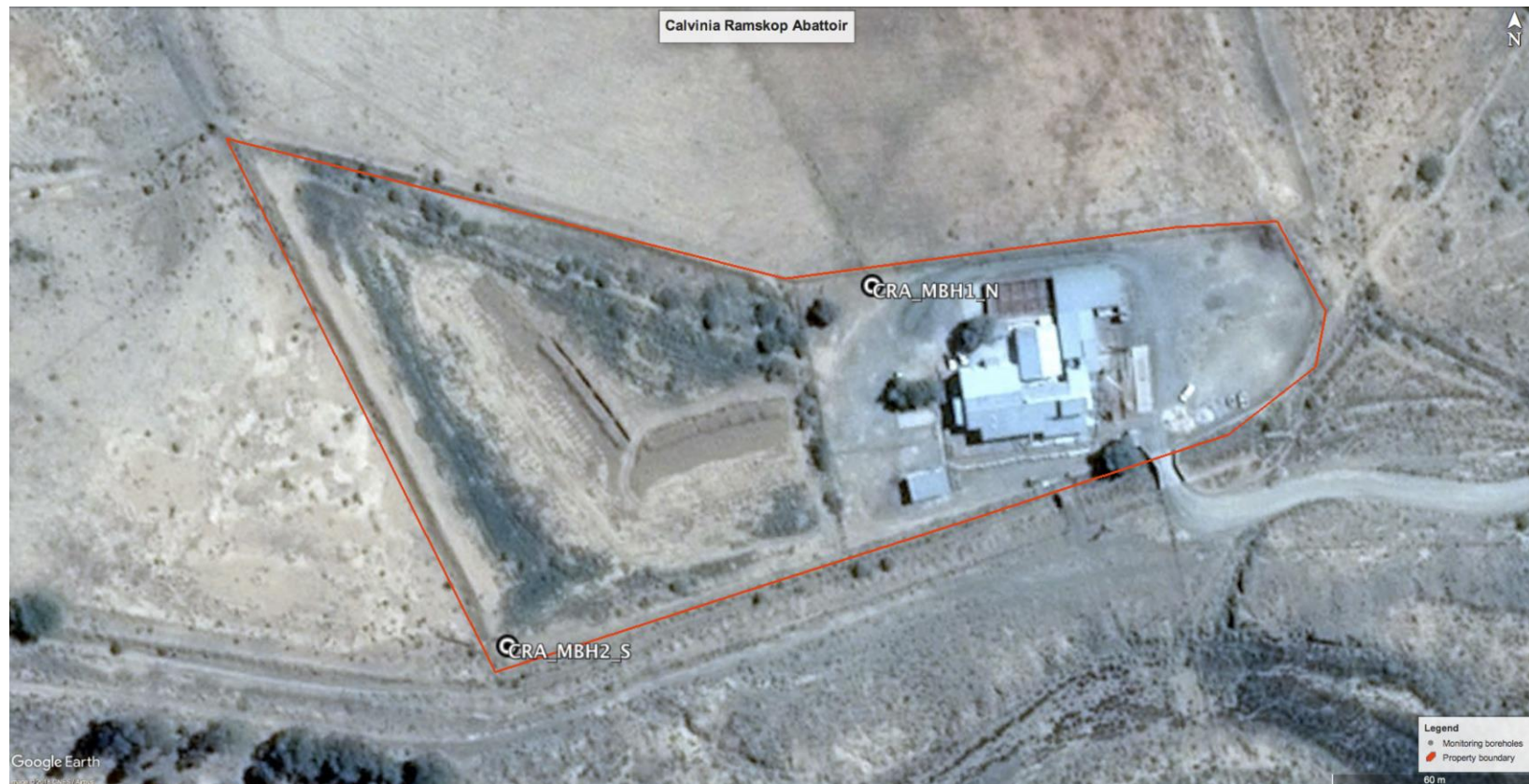
Figure 2: Monitoring borehole positions.
