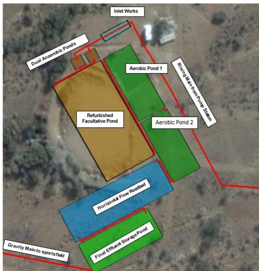
Figure 2: Proposed layout of refurbishment and improvement works of Klaarstroom WWTP (BVI Technical Report)
