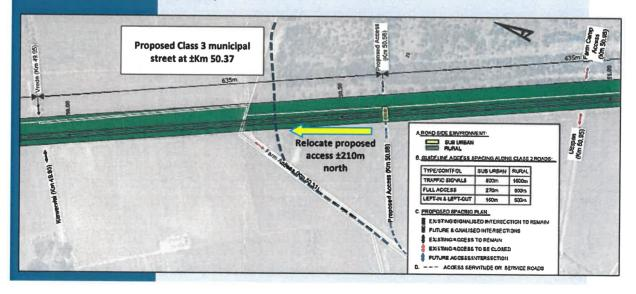
The farm access to the west of MR 174 at Km 50.31 will have to be realigned at the same time as the proposed access is implemented at Km 50.37.
