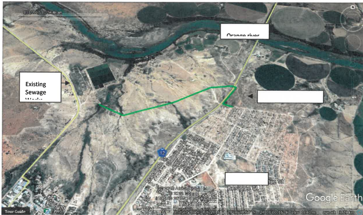
Figure 1: Google image indicating the proposed pipeline route in green, in proximity to Hopetown, the existing sewage works and the Orange River.
