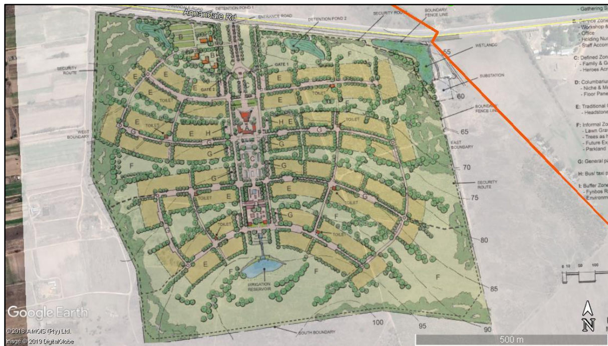
Figure 22: Georeferenced view of the preferred alternative layout. Note that the portion of Wetland B within the proposed site and its 15m buffer are rehabilitated as part of the parkland.
