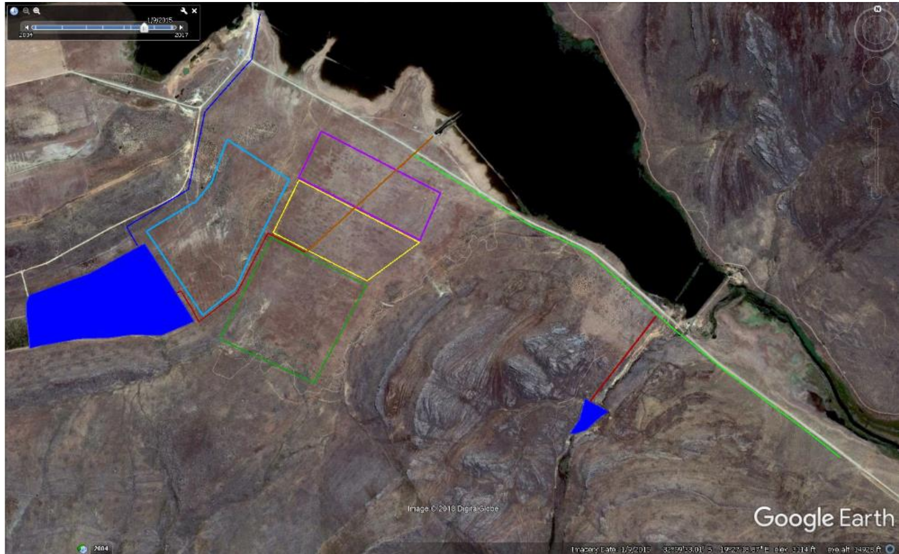
Figure 9: Google image indicating the proposed irrigation pipelines from the proposed Toeka dam (this application) and Harmony dam (separate application) to the proposed 75ha agricultural development. The red lines indicates the proposed new irrigation pipelines (both will be shorter than 1000m with a diameter smaller than 300mm). The brown and green lines indicates the existing irrigation pipeline routes.
