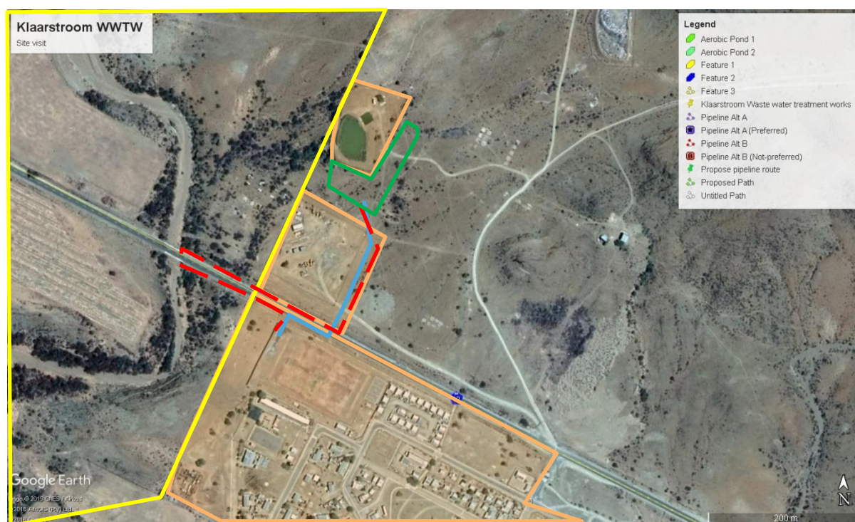
Figure 5: Google overview of the study area, showing the additional area that will be impacted by the proposed WWTW (green polygon), the preferred pipeline route in blue (as revised), the alternative pipeline route in red (as revised), in relation to areas that were basically transformed as a result of urban activities (in orange). The yellow area indicating private property.
