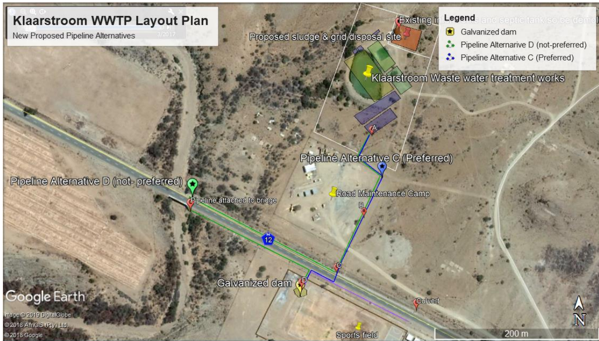
Figure 2: The location of the proposed Klaarstroom WWTW upgrades and potential pipeline routes (as revised)
