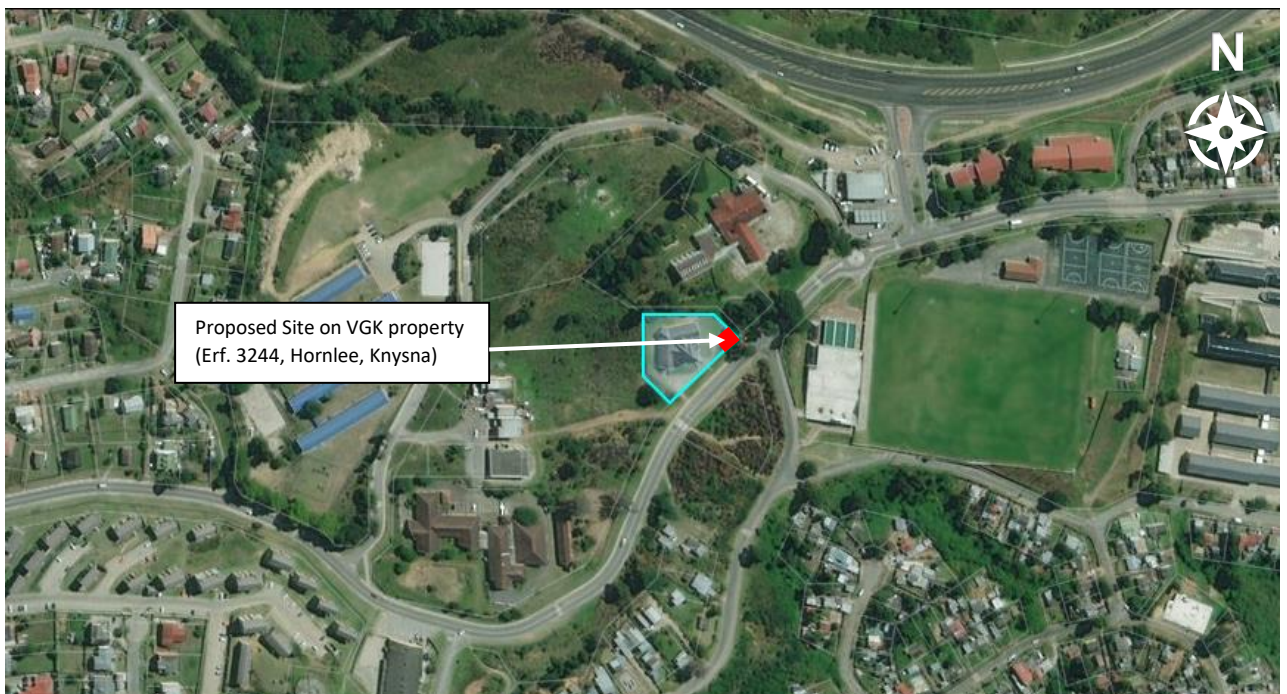
Figure 4: Proposed site for 25m high telecommunications monopole tree tower within VGK Knysna property off Vigilance Drive (corner of Erf. 3244, Hornlee, Knysna). Development footprint (approximately 10,6m x 10,6m or 112m 2 ) indicated in red.
