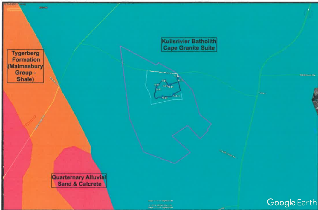
Figure 4. Geological map showing that the entire study area is underlain by the Kuilsrivier Batholith (Cape Granite Suite).
