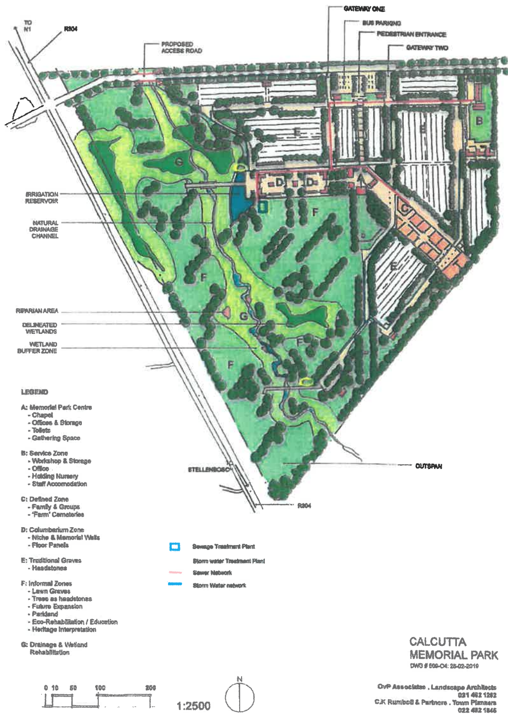
Figure 3: Storm water and sewage plan layout.
