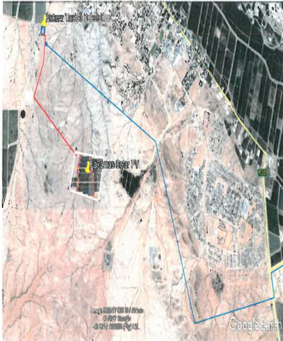
Figure 2 - position of the proposed project site and solar PV panel layout with nearby Eskom, Taaipit and smaller Hydro-SA substations (substation outlined in blue, proposed overhead power line tie-in for evacuation of electricity to Taaipit (Eskom) substation indicated in red. Existing overhead powerline servicing Hydro-SA and running within servitude 269/2013, indicated in light blue). Lighter red shaded area within proposed site indicates 32m setback from intermittent water courses running through proposed site
