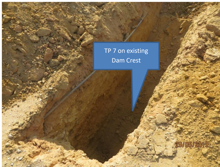
Figure 9: TP 7 Brownish-yellow clayey sand with gravel (existing dam core material)
