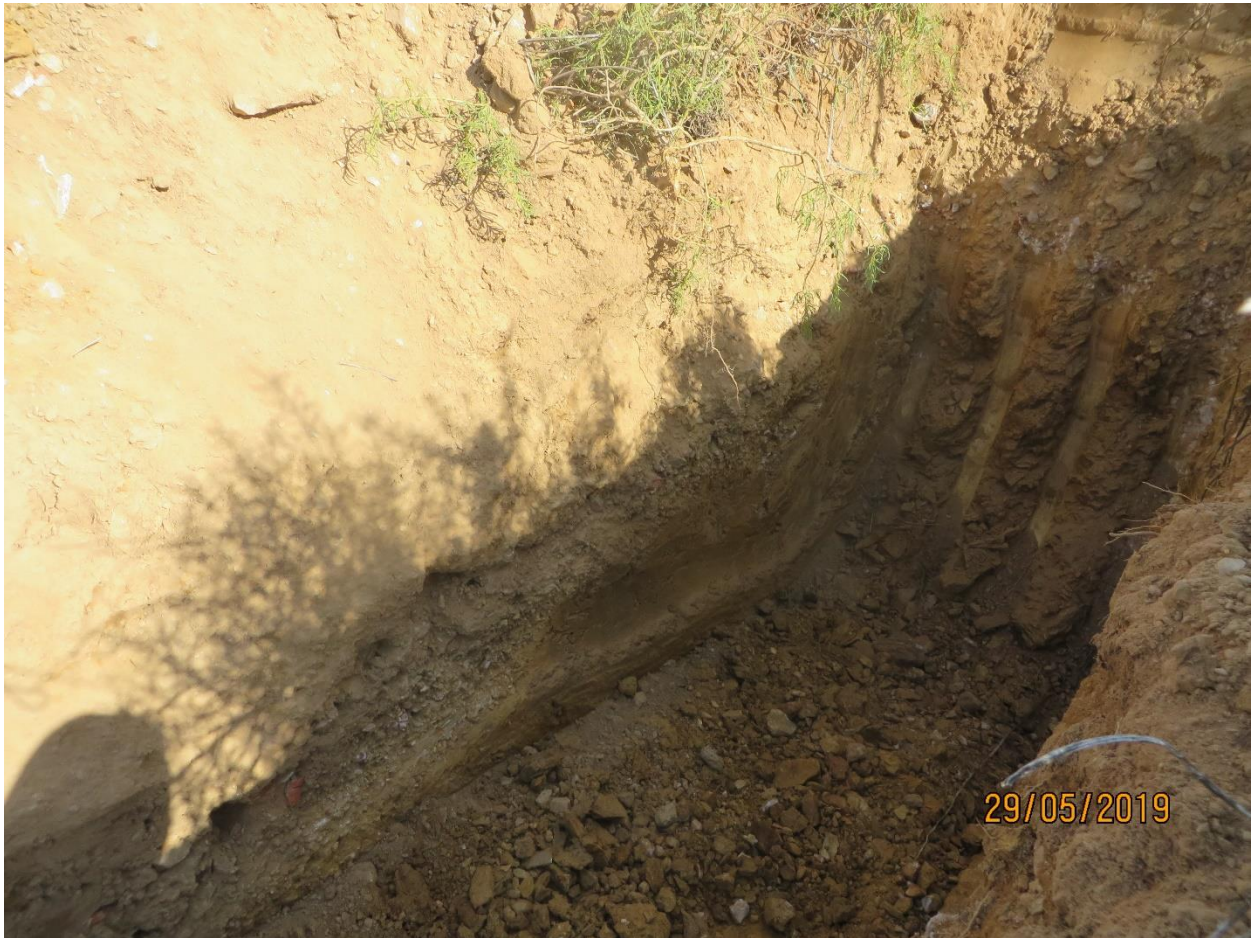
Figure 10: TP5- Brownish-yellow clayey sand with gravel located in the dam basin (proposed raising core material)
