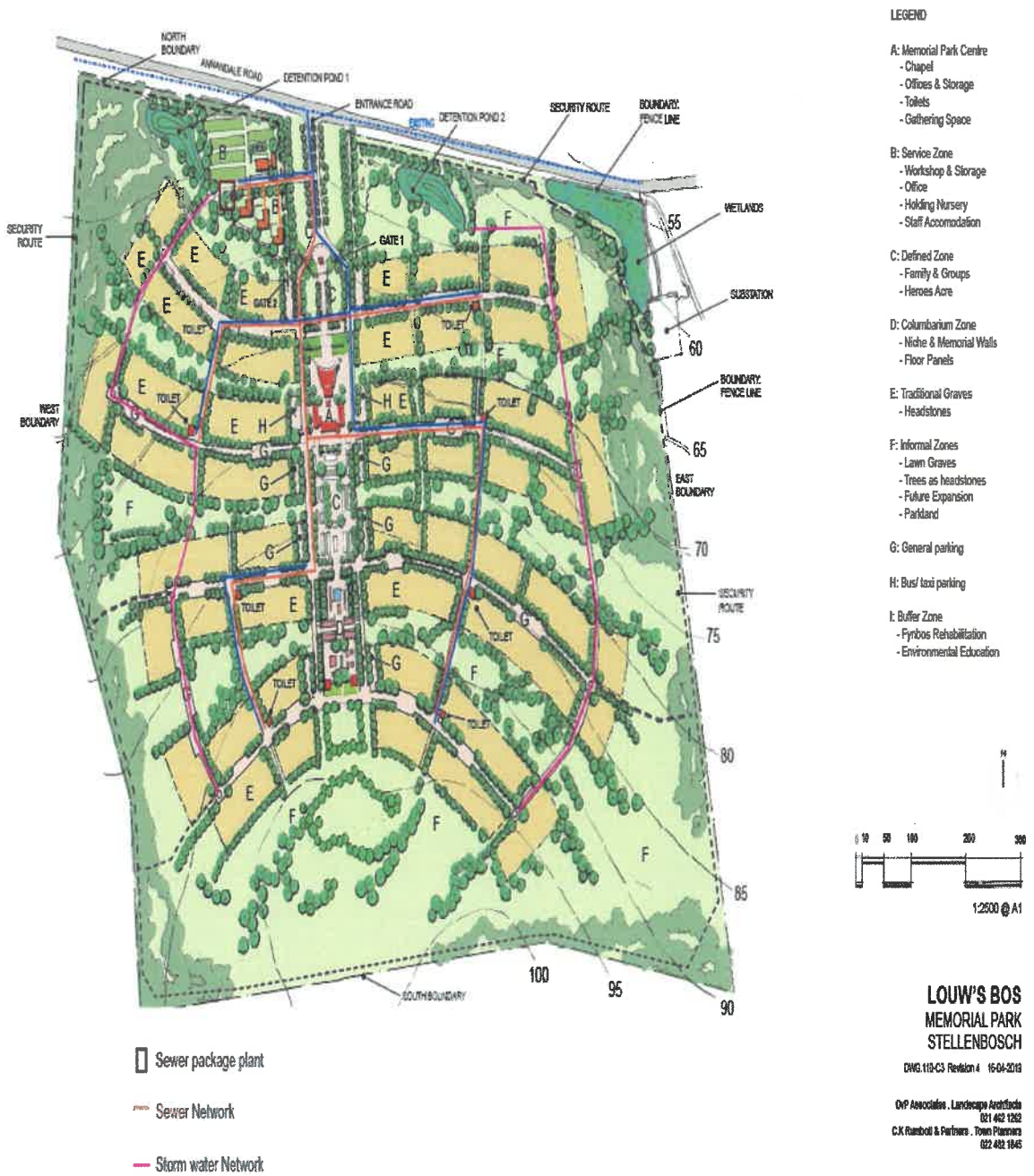
Figure 3: Storm water and sewerage plan layout.
