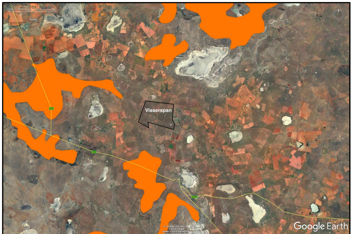
Figure 4. Geological map of Visserspan 40. The farm lies on sand over shale and mudstone (unshaded). The orange areas represent dolerite intrusions of which there are none significant at Visserspan 40.
