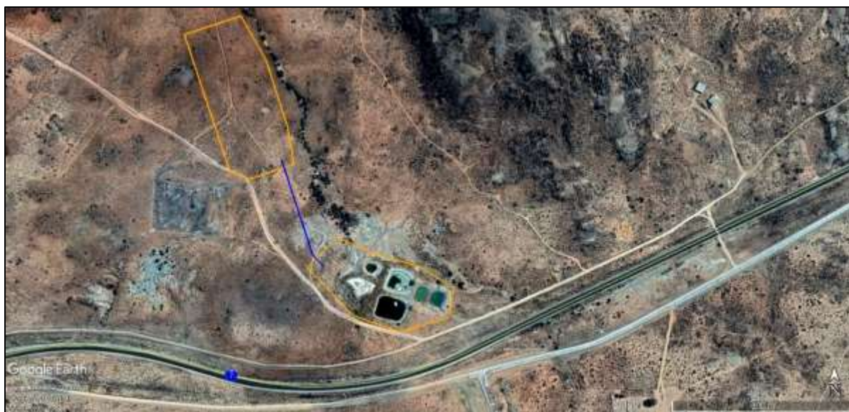
Figure 2: Close-up Google Earth© satellite image of the sewerage infrastructure project area with two sets of oxidation ponds surrounded by a fence (orange polygons) and joined by a pipeline (blue line).
