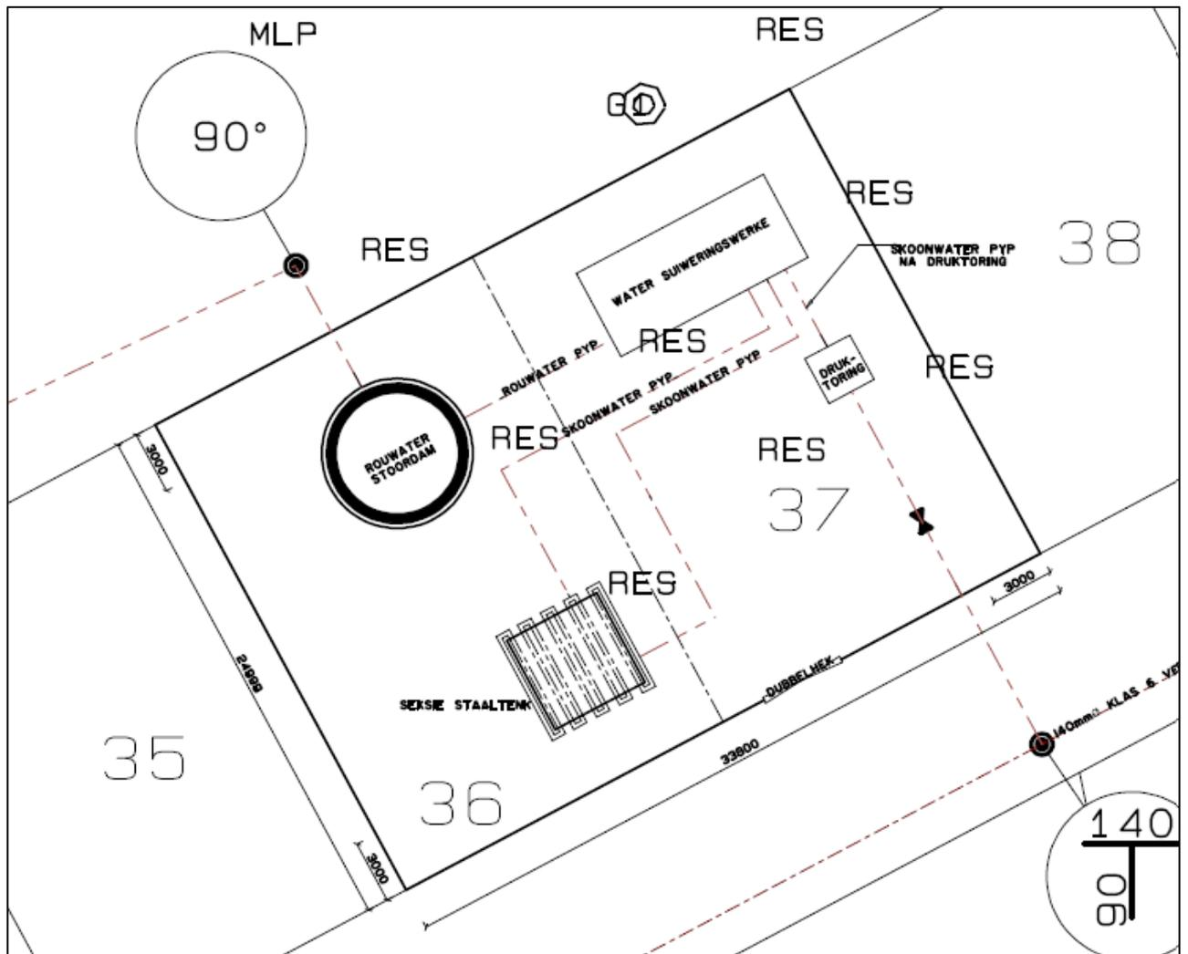
Water is pumped from the raw water storage dam through the Water Treatment Plant to a 110 m<sup>3</sup> sectional steel potable water storage reservoir. From there, it is pumped into the 10m<sup>3</sup> elevated storage tank before is gravitates into the village network.
