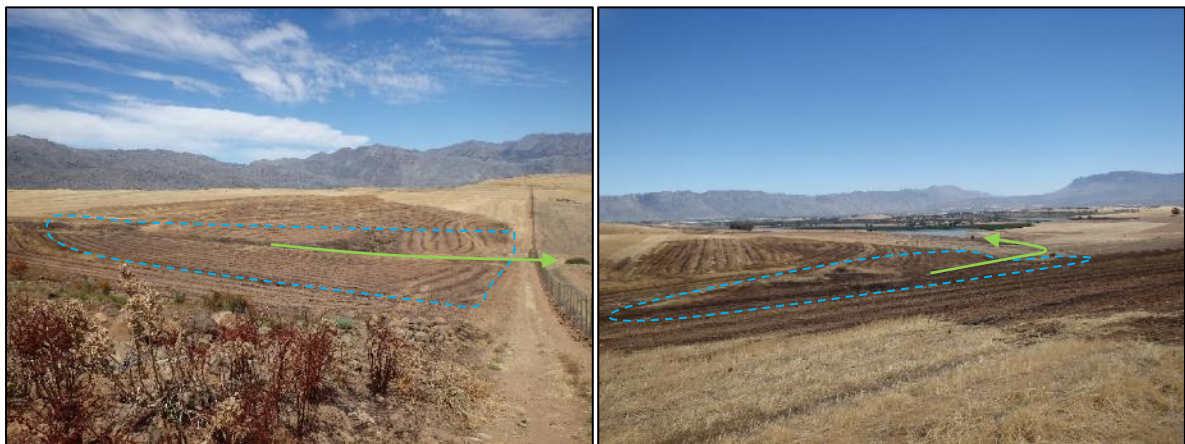
Figure 12: The blue line indicates the approximate extent of the footprint area of the proposed dam. The landscape position changes from a footslope (right) into a valley bottom position (left), draining in a south to north direction (green arrow).
