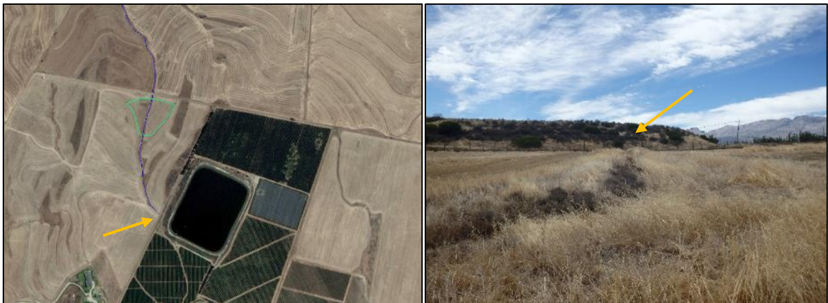
Figure 17: (Left) Digital satellite imagery indicating the most upstream point of the drainage line (yellow arrow) relative to the dam. (Right) It is clear that the drainage line is located just downstream of the dam, however, no evidence of seepage from the dam was evident.
