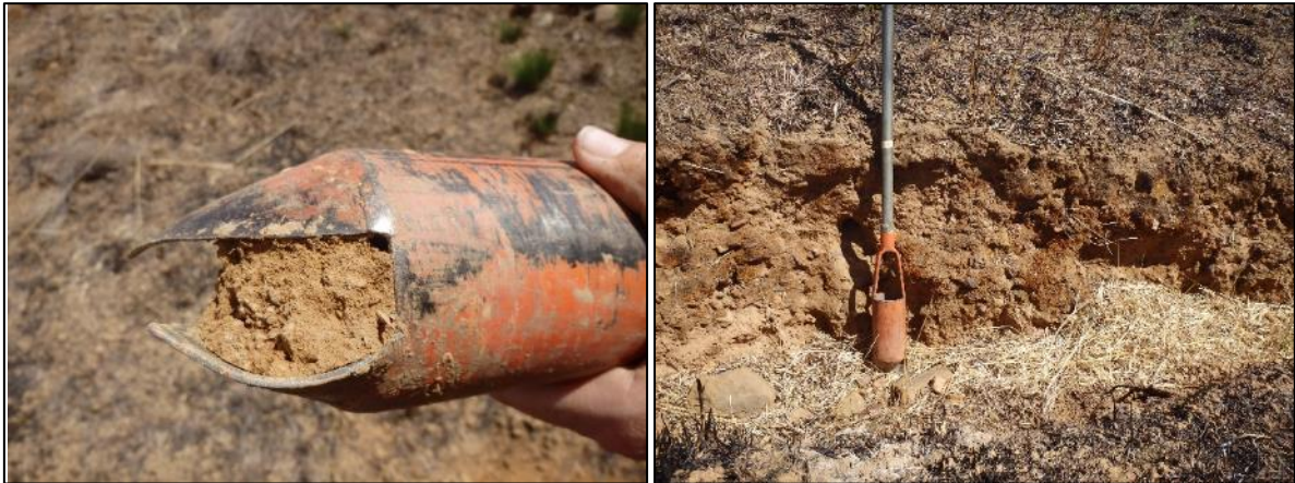
Figure 16: (Left) A hand auger sample, indicating uniform soil colour and strong structured soil. (Right) The soil profile of the erosion gully is rocky did not show any variation in colour or structure.
