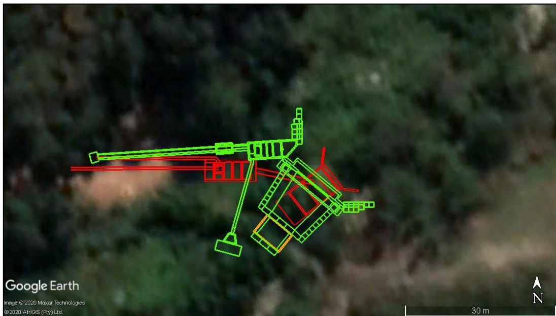
Figure 3. Overlay of previously authorized water structure (outlined in red) and proposed amendment to water structure (outlined in green). Note, gabions are depicted on the proposed amendment whereas associated erosion-protection infrastructure is not depicted for the previously authorized water structure. The amended water structure footprint will also include the construction of temporary, low-flow diversion channel which will direct clean stormwater around the works by the furrow berm as well as a temporary berm and cut-off upstream of the proposed water structure during the construction phase (please refer to Appendix G). This will reduce erosion and sedimentation associated with construction activities. Hay Bale-Bidim-Shade cloth filter structures will also be placed downstream of the water structure to reduce downstream erosion / sedimentation. As per the overlay image above, the location of the area which will be disturbed by either water structure are similar.
