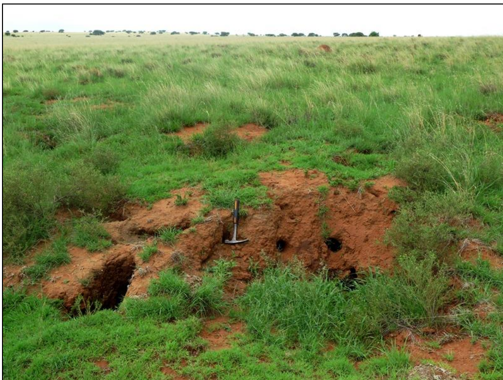
Figure 19: Thick, orange-brown sandy soils overlying dolerite, Solar PV 1 project area (Hammer = 30 cm). The soils are extensively burrowed here.
