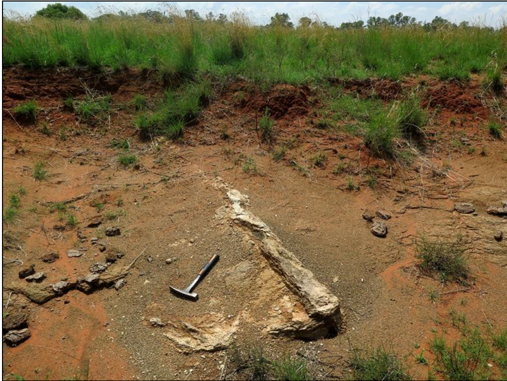
Figure 8: Weathered dolerite on margins of borrow pit situated on the south-western edge of Solar PV 4 project area showing a thick inclined vein and sheet of subsurface calcrete (Hammer = 30 cm).
