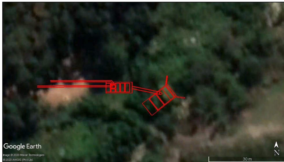
Figure 1. Previously authorized water structure as per the Environmental Authorisation. It must be noted that the permanent footprint for the water structure is \pm 430\text{m}^2 where the total area to be cleared for construction activities will be 558\text{m}^2 of which 128\text{m}^2 will be rehabilitated post-construction. Moreover, as part of construction activities, the areas surrounding the authorized structure would be disturbed and subsequently rehabilitated post-construction. Erosion mitigation measures associated with the structure, required to stabilize the banks, are not depicted in the figure above.
