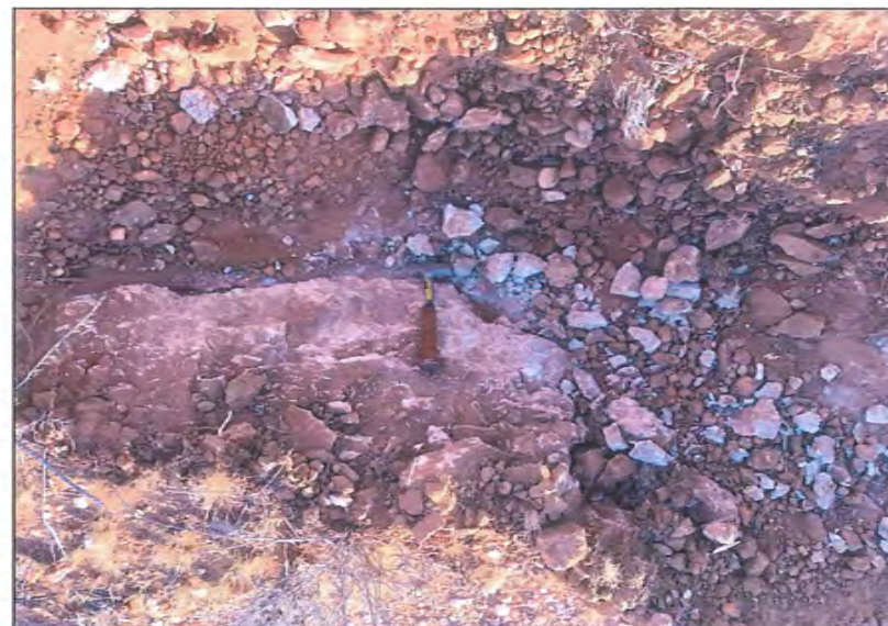
CONDITIONS OF HARD EXCAVATION IN CALCRETE
