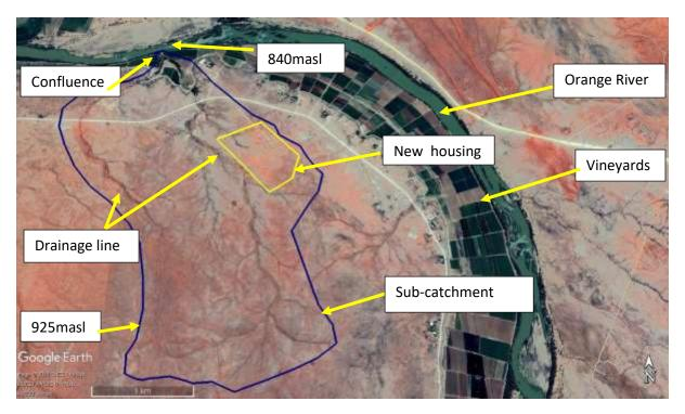
Figure 7 Opwag housing and drainage line
