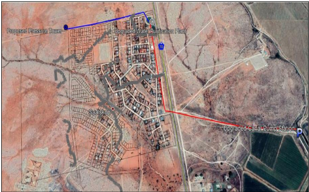
Figure 23. Graphical representation of required water supply upgrades. Engineer's Service Report (Appendix 4B).
