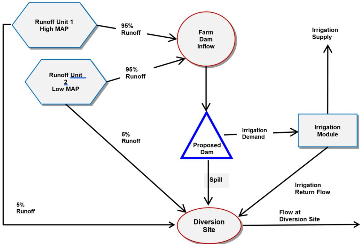
Figure 2.3 Configuration diagram of the Pitman model for the proposed dam catchment.
