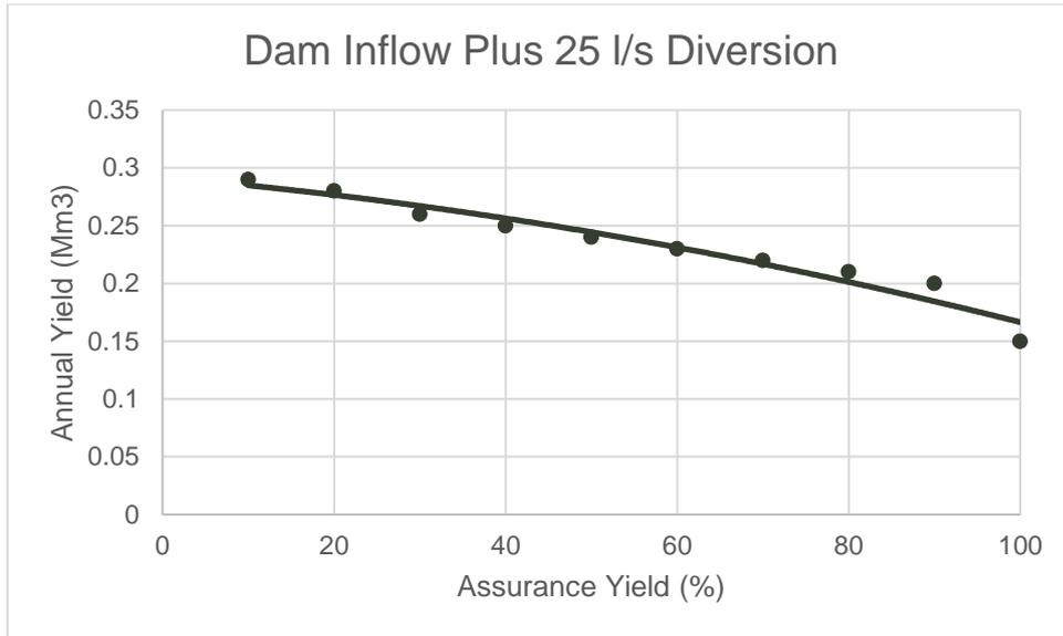
**Figure 4.3** Proposed Dam yield (Mm<sup>3</sup>/ann) using upstream inflow and diversion with a pumping capacity of 25 l/s.
