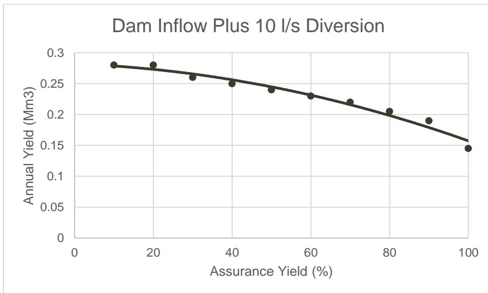
Figure 4.2 Proposed Dam yield (Mm<sup>3</sup>/ann) using upstream inflow and diversion with a pumping capacity of 10 l/s.
