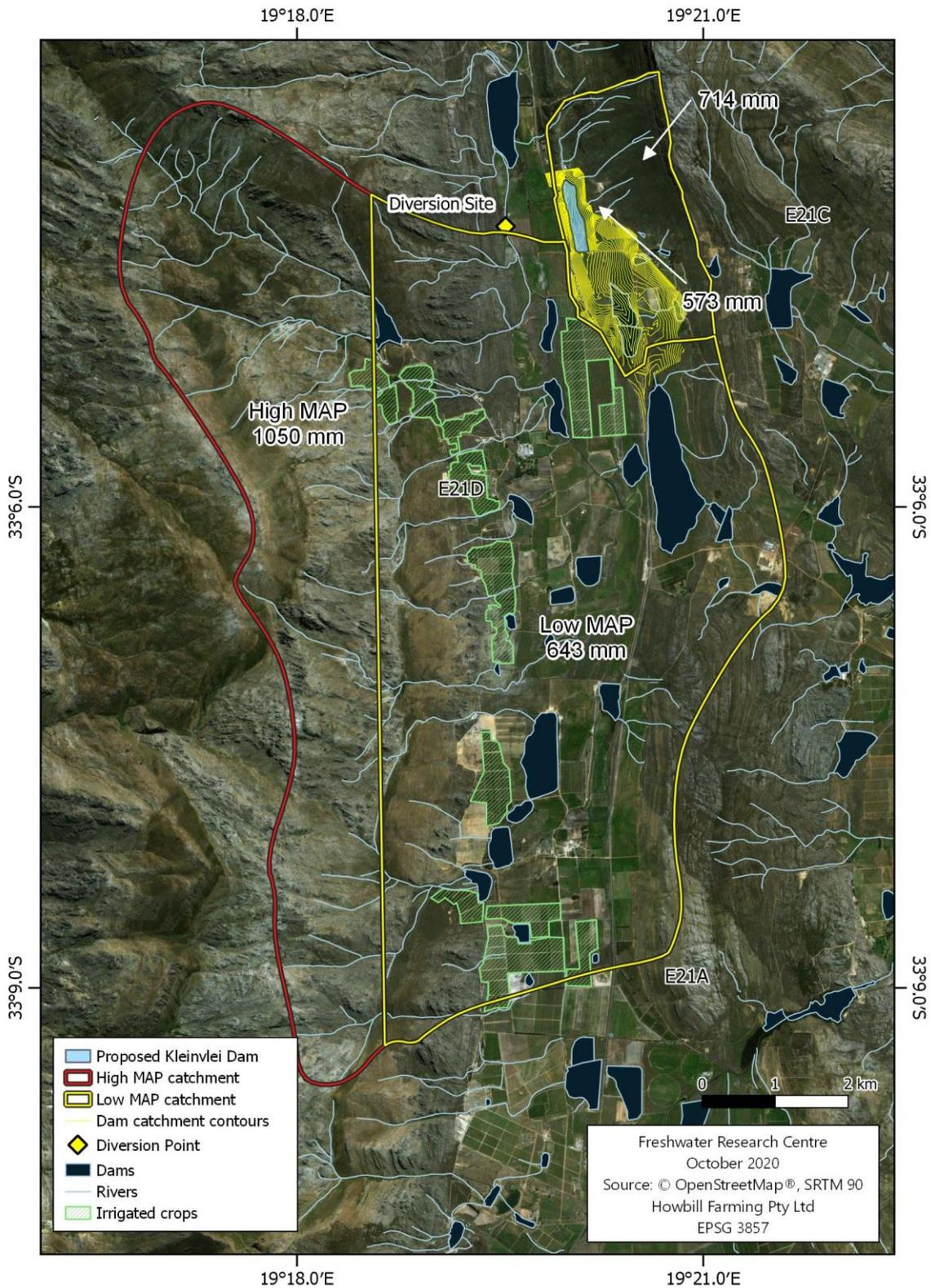
**Figure 2.2** Location of the proposed Kleinvlei Dam and supplementary Diversion Site with catchment boundaries delineated for each. High Mean Annual Runoff (MAP) and Low MAP areas are shown as well as the Kleinvlei Dam catchment and irrigated crops.
