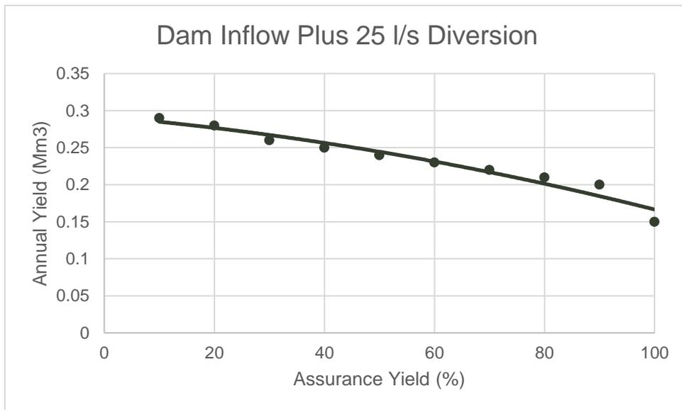
**Figure 4.4** Proposed Dam yield (Mm<sup>3</sup>/ann) using upstream inflow and diversion with a pumping capacity of 50 l/s.
