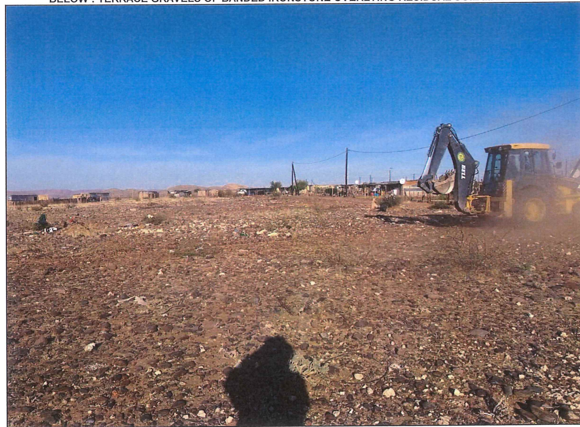
TOP : STEEPLY DIPPING QUARTZ-MUSCOVITE SCHIST BELOW : TERRACE GRAVELS OF BANDED IRONSTONE OVERLYING RESIDUAL SOIL MATERIALS
