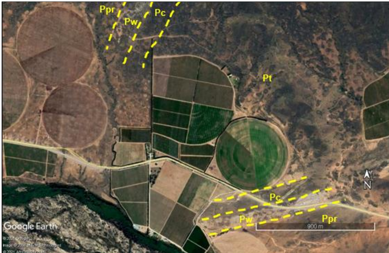
Figure 15. Google Earth© satellite image of the project area north of the Breede River. The small agricultural project areas (A, B) are underlain by the Collingham and Tierberg Formations (Pc, Pt) while the in-stream dam site lies within the Tierberg outcrop area (Compare Figures 2 & 3). Direct impacts on the palaeontologically sensitive Whitehill Formation (Pw) and Prince Albert Formation (Ppr) are not anticipated here.
