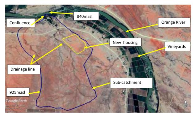
Figure 7 Opwag housing and drainage line
