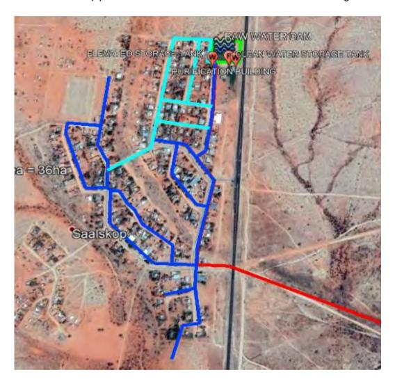
Figure 5 The reticulation network
