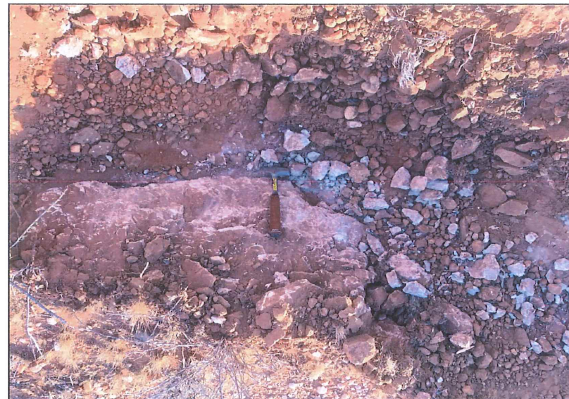
CONDITIONS OF HARD EXCAVATION IN CALCRETE
