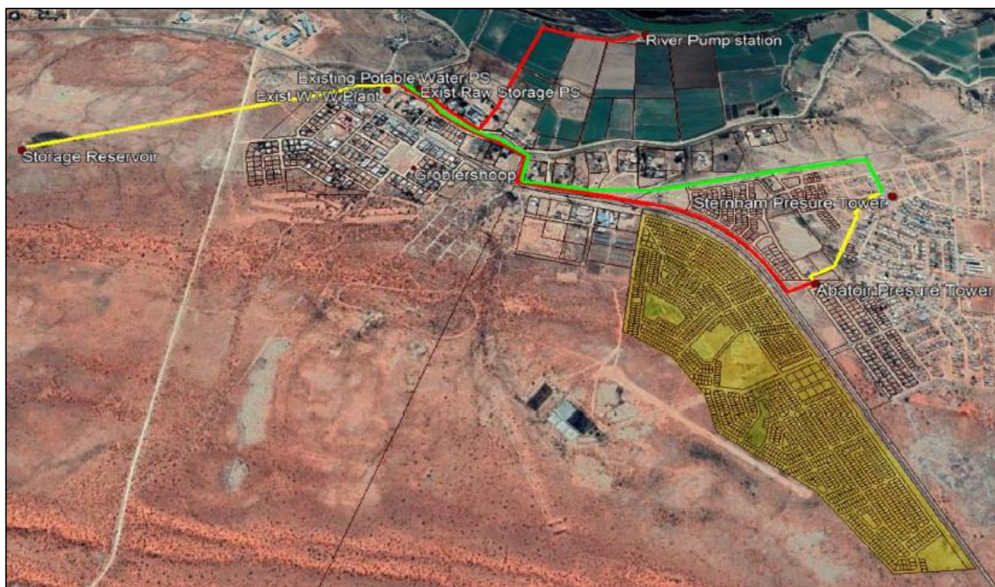
Figure 25. Current bulk water supply and water reticulation. Source: Engineer's Service Report (Appendix 4B).
