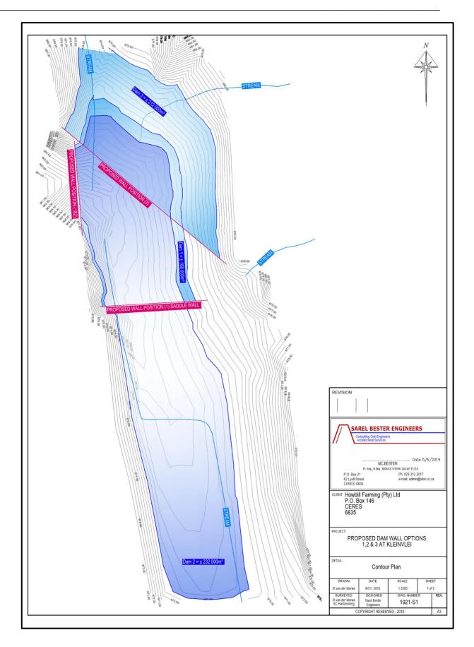
Figure 3. Engineers' drawing of the alternatives for the proposed Kleinvlei Dam.
