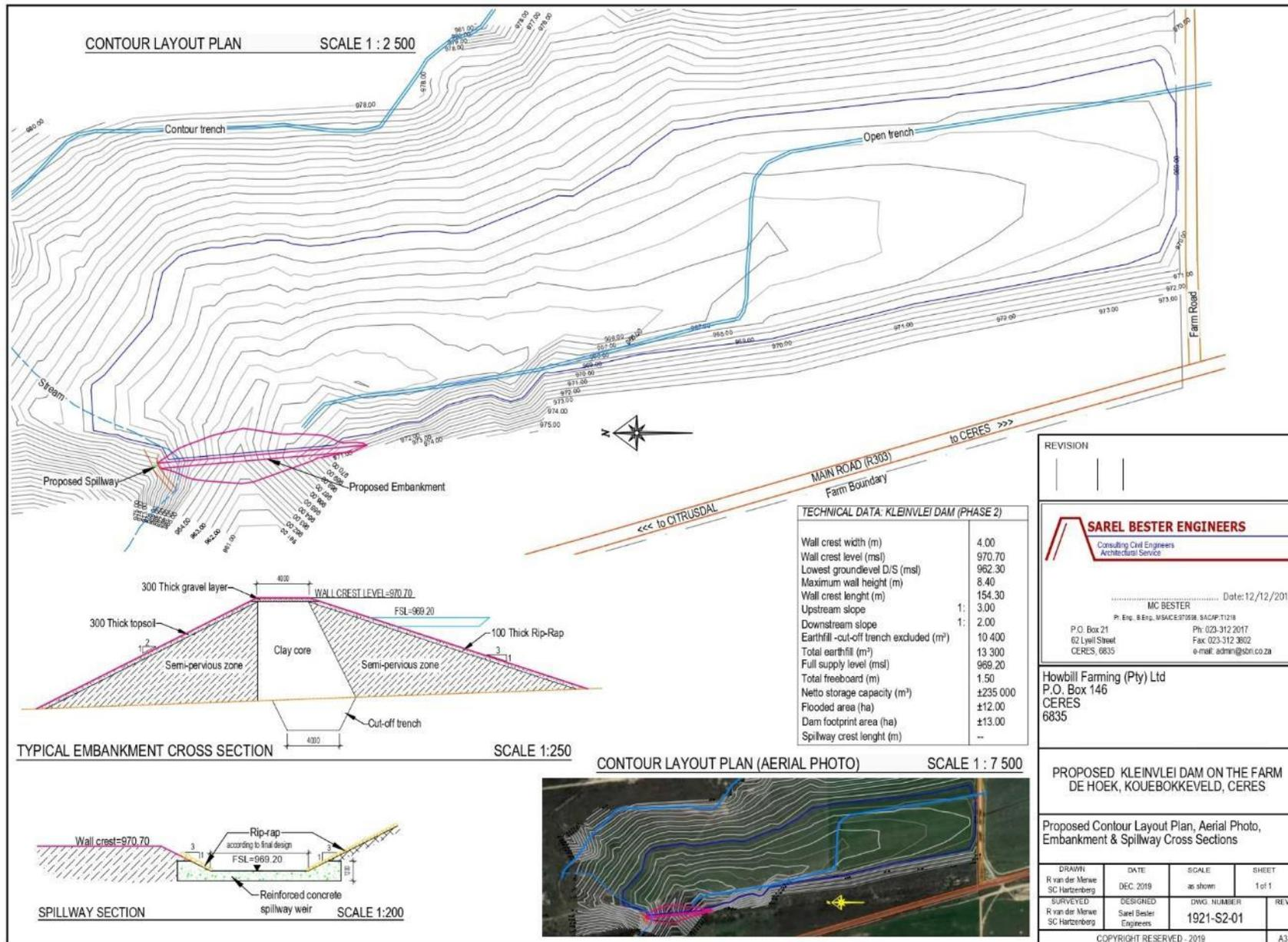
Figure 3: Proposed design of the Kleinvlei Dam (Sarel Bester Engineers, 2019).
