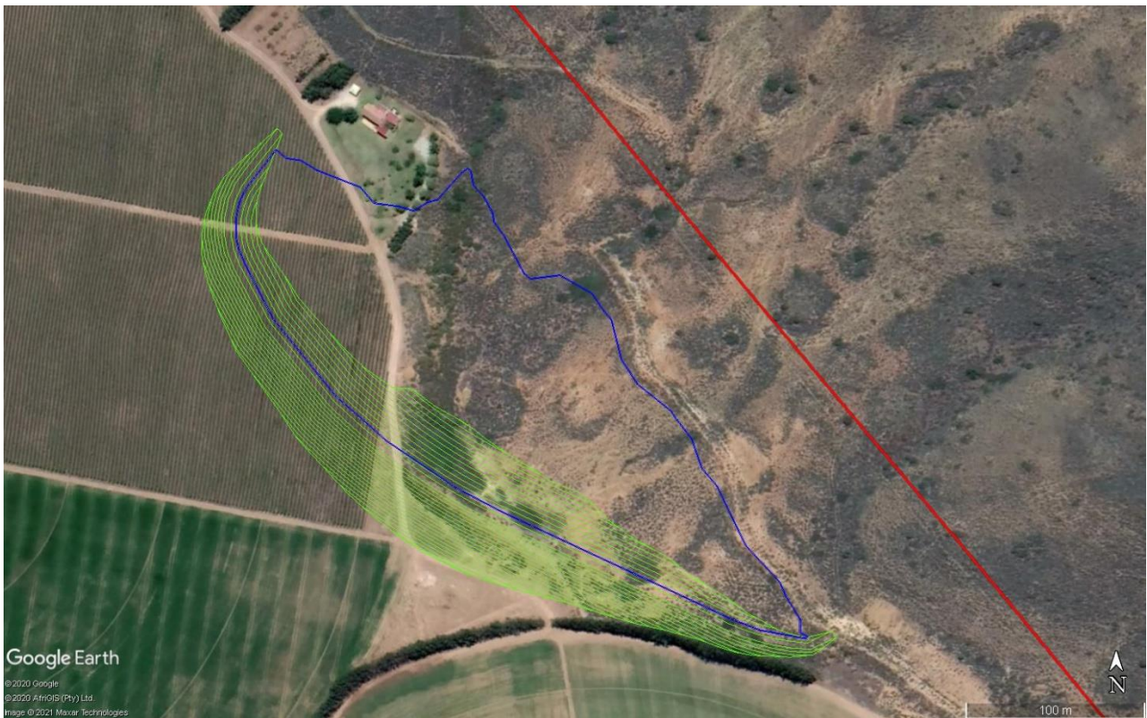
Figure 3: GOOGLE EARTH IMAGE INDICATING THE PROPOSED DAM. THE GREEN AREA SHOWS THE DAM WALL FOOTPRINT, AND THE BLUE LINE THE HIGH-WATER MARK OF THE DAM.
