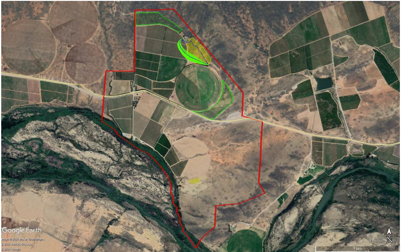
Figure 3: GOOGLE EARTH IMAGE INDICATING THE PROPOSED DAM. THE GREEN AREA SHOWS THE DAM WALL FOOTPRINT, AND THE BLUE LINE THE HIGH-WATER MARK OF THE DAM.
