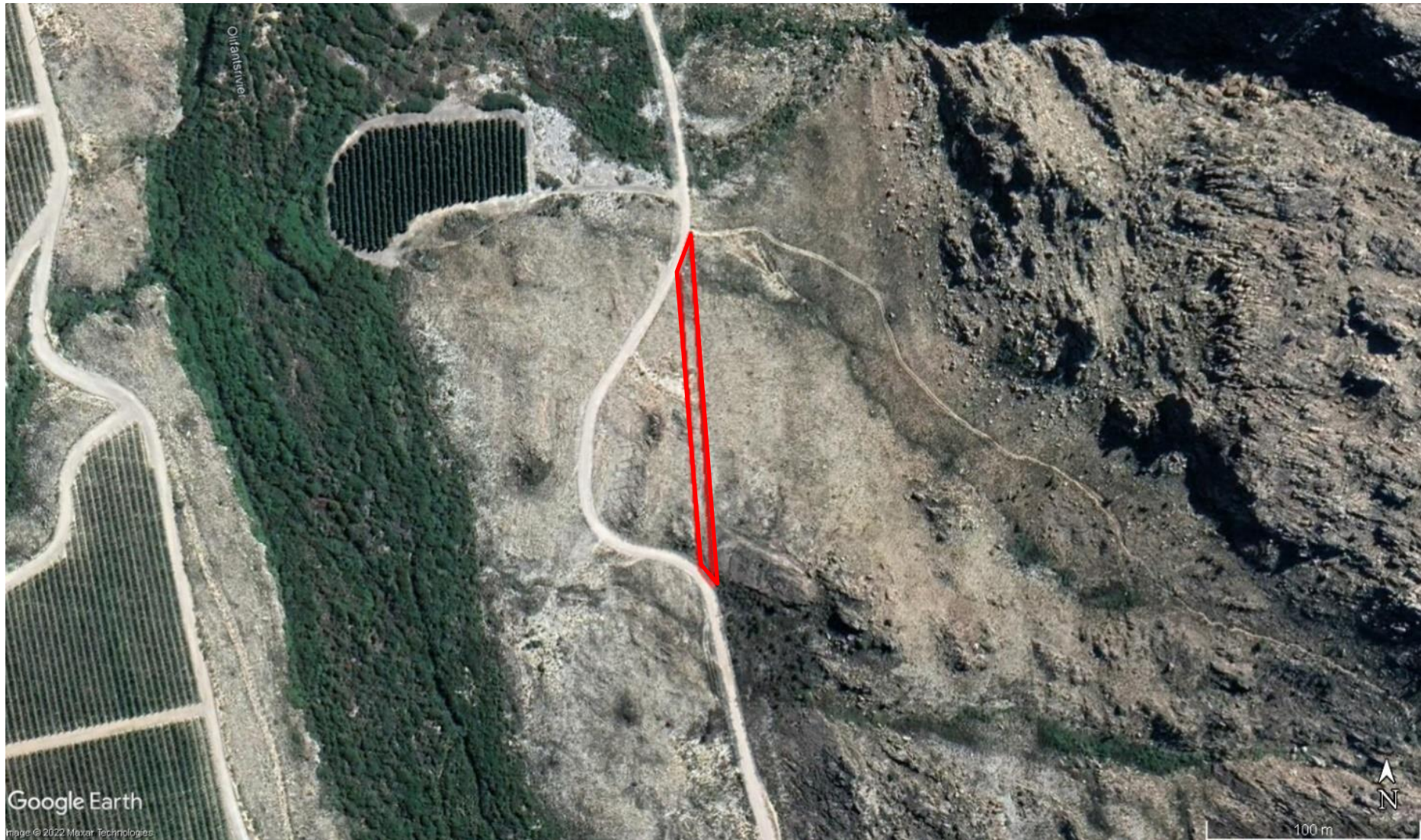
Figure 6: Google Earth Image indicating the realignment of road section 1.
