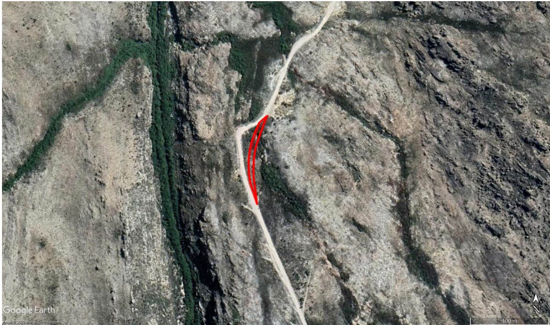
Figure 8: Google Earth Image indicating the realignment of road section 3.
