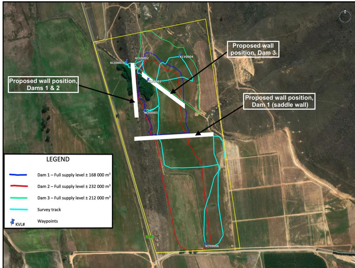
Figure 7. The proposed dam alternatives superimposed on a Google Earth™ image together with the survey track and waypoints.
