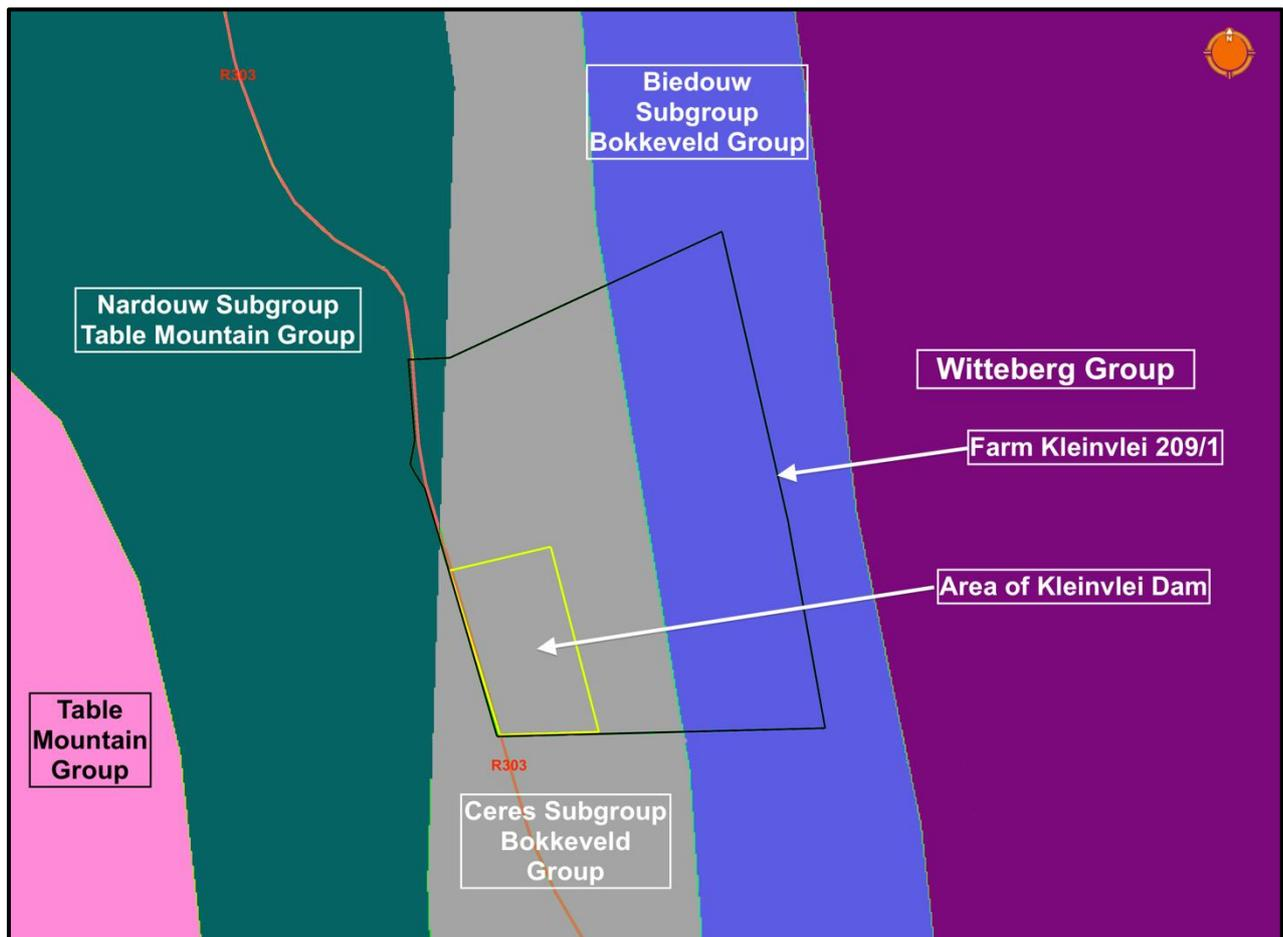
**Figure 4.** Geological map from 1: 1 000 000 shapefiles from Geological Survey, superimposed on a Google Earth™ image. The Kleinvlei Dam would be located on shales of the Ceres Subgroup and marginally on sandstone of the Nardouw Subgroup.
