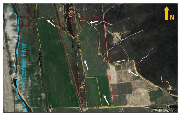
Figure 7: Digital satellite imagery (2019) of the locality of the excavated channels (yellow lines) in the study area (red outline). The purple dashed lines depict episodic drainage lines conveying surface runoff from the mountainous area into the excavated channels.
