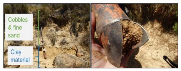
Figure 13: (Left) the soil profile of an ephemeral drainage line. (Right) A soil auger sample taken in the episodic drainage line indicates the deposition of fine alluvium material with round cobbles.
