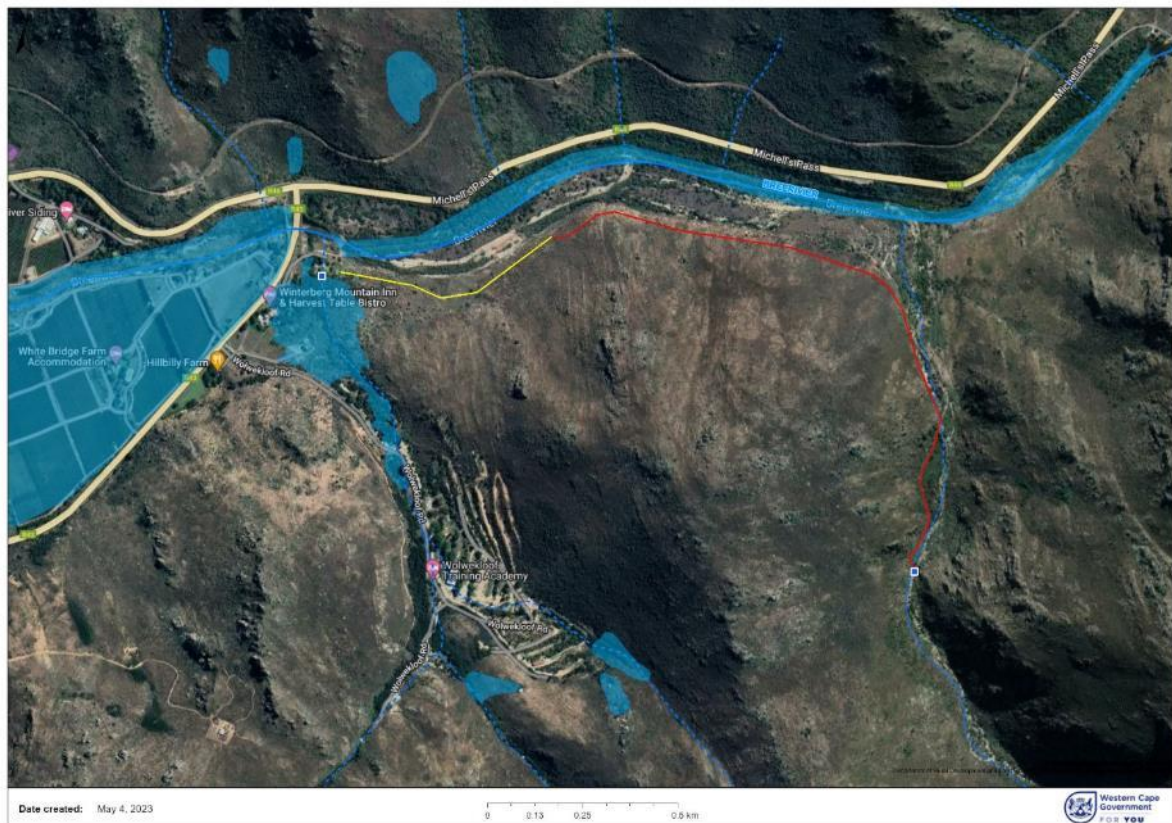
Figure 3: A google image showing the pipeline route: Yellow = underground section; Red = aboveground section.
