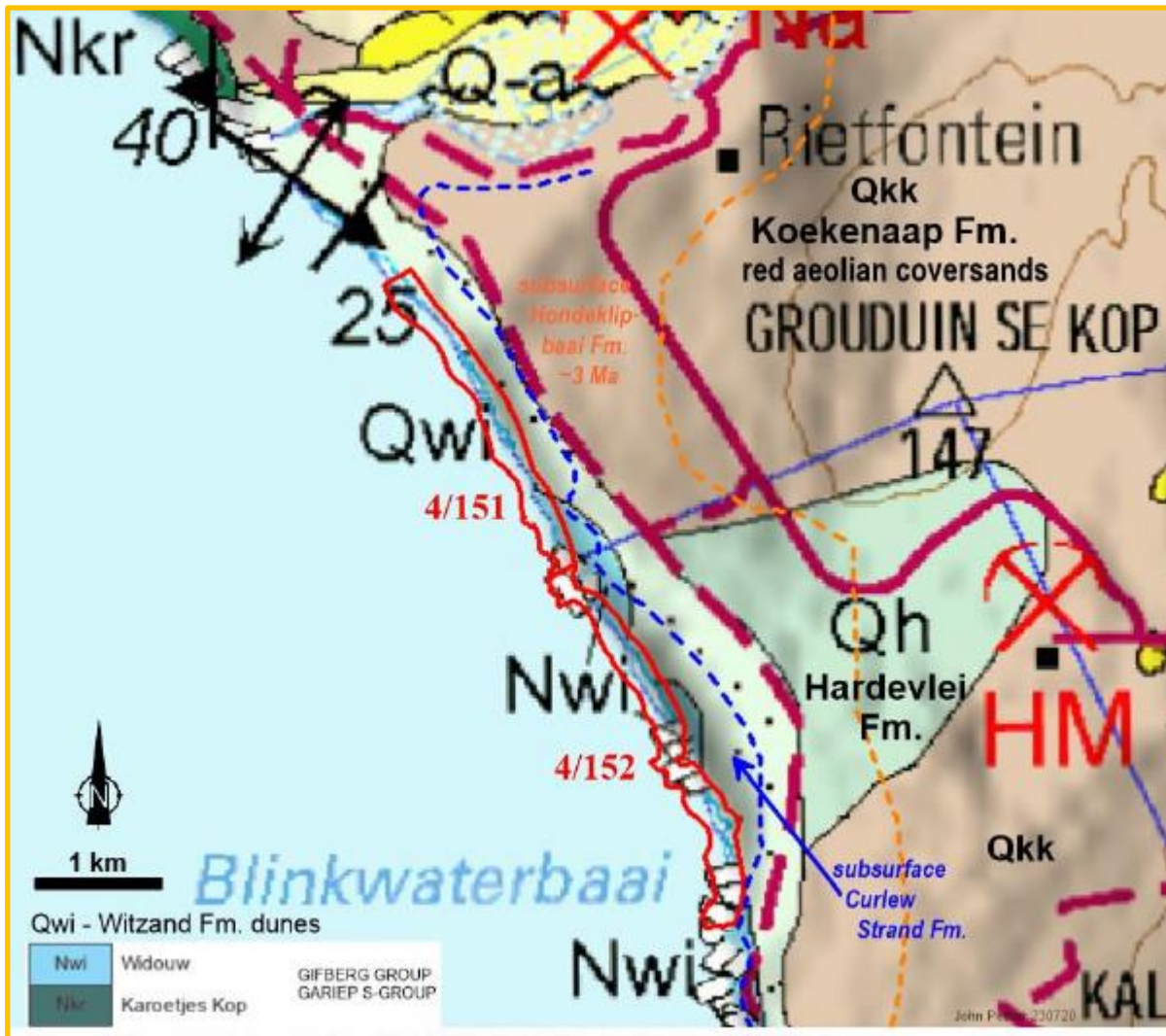
Figure 6b: Surface geology of proposed site with approximate subsurface extent of underlying marine formations
